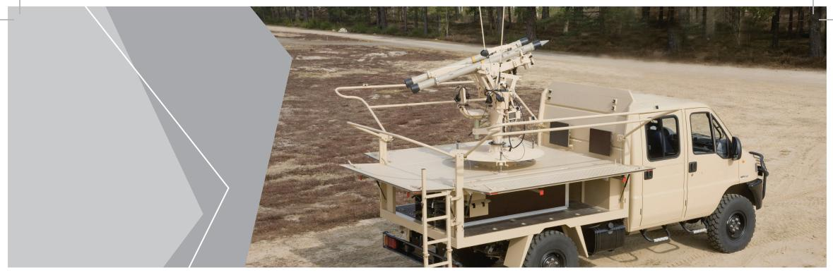
MISTRAL ATLAS is a very short range air defence weapon system, firing the MISTRAL, latest generation fire-and-forget missile.
