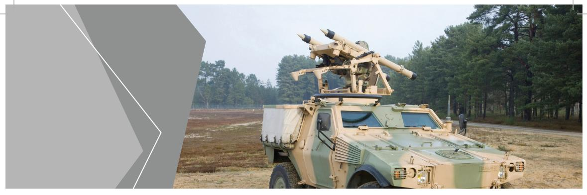
MISTRAL ALBI is a lightweight, 360° turret, optimised for the protection of armoured or mechanised units as well as convoys and which, additionally, provides crews with an excellent level of protection
