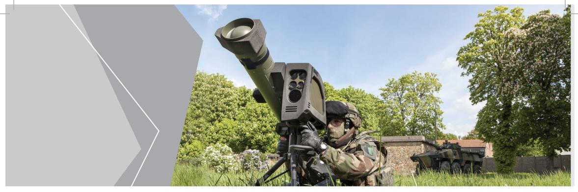
The latest (fifth) generation land combat missile system designed for dismounted infantry as well as for integration on combat vehicles. Featuring both fire-and-forget and man-in-the-loop operation, network-enabled MMP also receives third party target designation for indirect firing scenarios.
