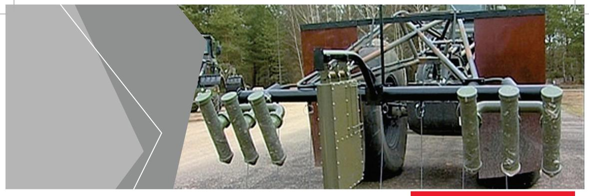
DEDALE is a unique off-the-shelf decoying system designed to be compatible with and to complement other mine clearing systems such as rollers, ploughs and flails. Easily installed on mine clearing vehicles, DEDALE activates all types of magnetic mines at a safe forward distance by transmitting a programmable decoy magnetic signature. Operating at normal column speed, DEDALE offers optimum levels of protection to route clearing systems such as SOUVIM 2.
