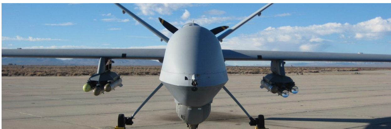
BRIMSTONE substantially increases persistence through single shot precision, 3 missile per pylon aerodynamic fit, and fast-jet qualified levels of environmental robustness
