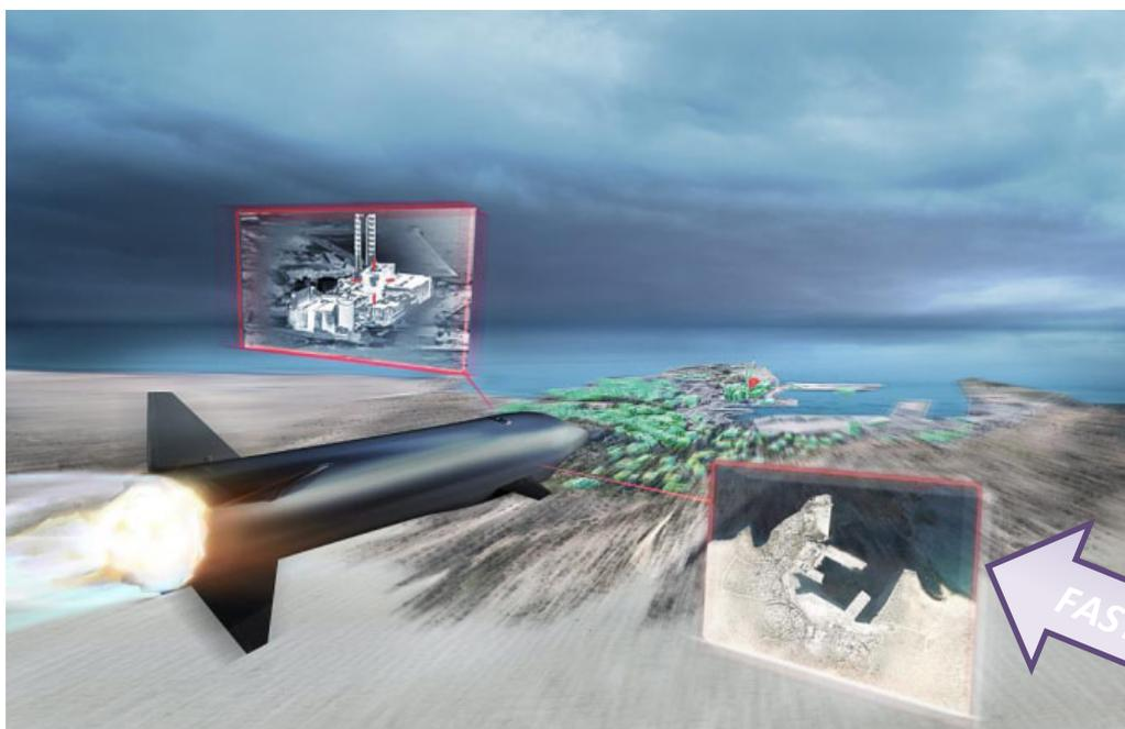
*Novel target matching technique - allows designation images (such as those from visible-band satellites) to be correlated with on-board seeker images (such as IR) despite differences in viewpoint and frequency band. This enables a significant reduction in the engagement timeline and allows more flexibility and robustness to changing conditions.*
