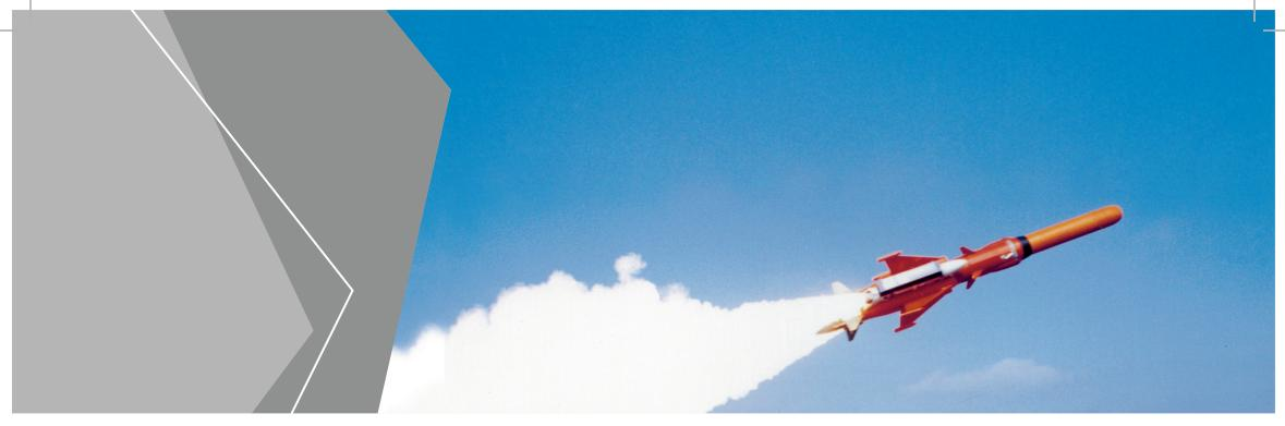
Derived from the OTOMAT MK2 missile system, MILAS is designed to carry and release an MU-90, or similar, lightweight torpedo, close to the designated submarine position, as indicated by the ship sonar or by a co-operating ASW helicopter or MPA.
