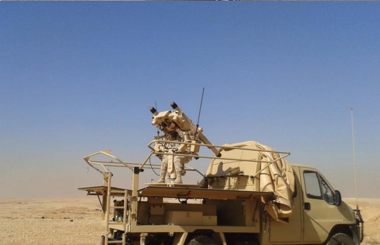
ATLAS is a twin manual MISTRAL missile launcher, which can be mounted on vehicle or easily deployed on ground. ATLAS is extremely easy to operate with its missile fire-and-forget system, much like the single missile launcher, MANPADS. The gunner simply needs to detect the target through the thermal sight, activate the MISTRAL seeker and fire after the missile is locked on the target.
