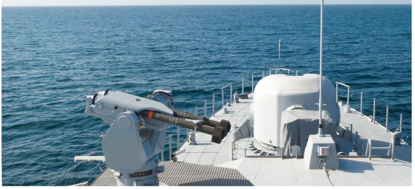
MISTRAL SIMBAD-RC is an anti-air self defence system operating the very effective fire-and forget MISTRAL missile. The system provides an extremely effective defence capability against all threats (anti-ship missiles, aircraft, helicopters as well as asymmetric surface threats). It has been optimised to handle a multi-threat scenario.
