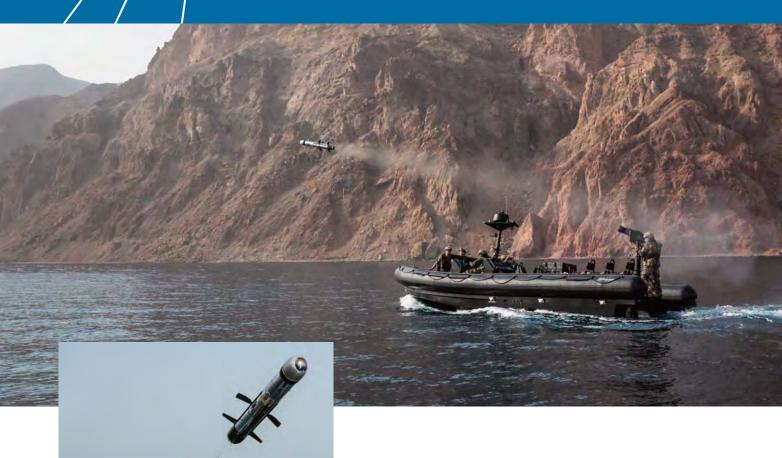
AKERON MP can provide a number of solutions for naval platforms including RHIBs (Rigid Hulled Inflatable Boats) and USVs (unmanned surface vessels). The land system firing post needs only to be inserted into a suitably positioned mount which can be easily retrofitted onto RHIBs and other small craft.
