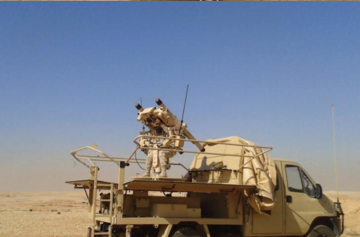
ATLAS is a twin manual MISTRAL missile launcher, which can be mounted on vehicle or easily deployed on ground.
