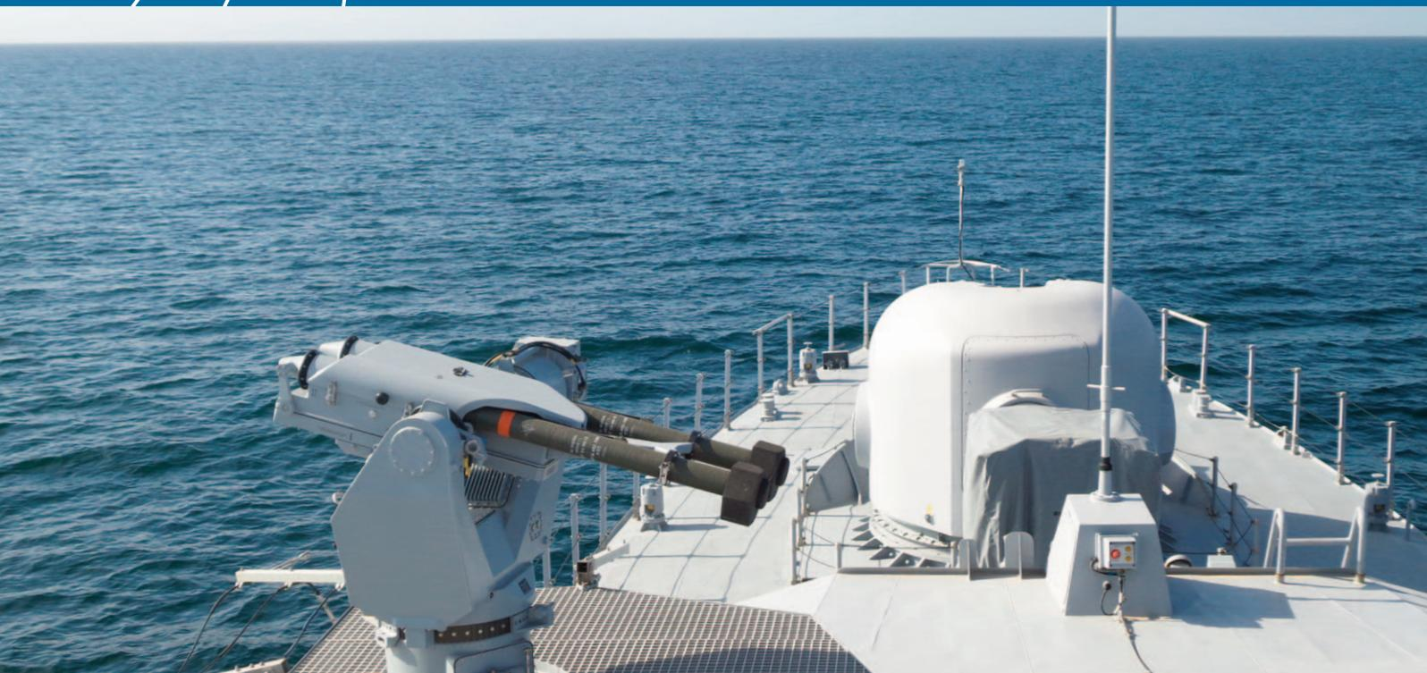
MISTRAL SIMBAD-RC is an anti-air self defence system operating the very effective fire-and forget MISTRAL missile.
