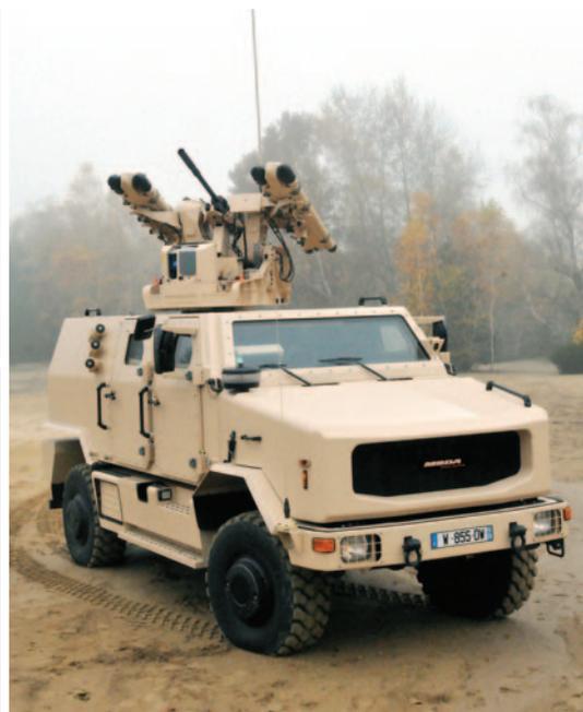
In addition to an autonomous IFF, MPCV uses a first class suite of gyrostabilised electro-optic sensors, which includes TV and IR sights, laser range-finder and automatic tracker. The system can operate both day and night and fire on-the-move thereby enabling it to carry out convoy escort missions or to provide mobile protection of deployed mechanised/armoured units with an outstanding degree of effectiveness.
