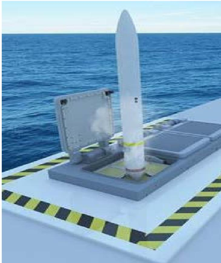
**Caption:** An MBDA Common Anti-air Modular Missile is ejected from a Lockheed Martin 3-Cell ExLS Launcher. The launcher, which is scheduled to be available in 2016, is designed for smaller Navy platforms that cannot accommodate the flexible 8-cell MK41 Vertical Launch System.
