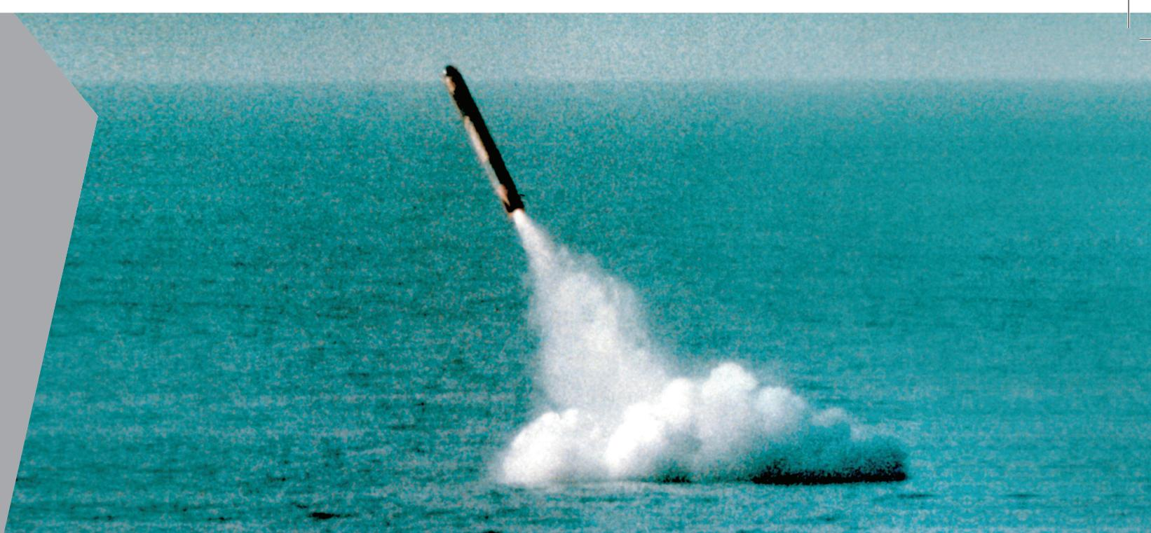
EXOCET SM39 is the submarine-launched version of the EXOCET family. It features all weather capability, sea skimming flight, solid propellant and a high kill warhead.
